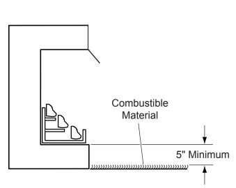
Figure 7 - Minimum Clearance above Combustible Flooring
